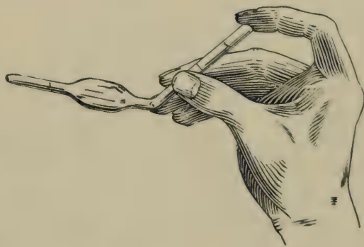
Fig. 36. Position of Weighing Pipette Before Placing in Holder.
